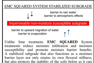
barrier layer not only retains its own flexural stiffness, but also protects the stability of the soils below as it cuts off the atmospheric effects (wetting and evaporative) and fluctuations in moisture content that otherwise drive the swelling and shrinking in the soils below the treated subgrade and generate differential settlement, roughness and cracking in the pavement above.
