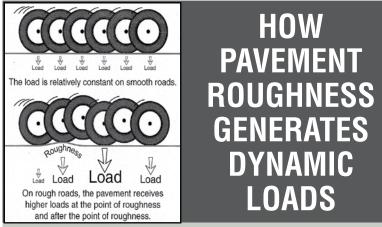
Pavement roughness leads to higher dynamic loads on localized pavement sections which increases pavement deterioration at those locations. This not only lowers ride quality, but also leads to a cycle of increasing deterioration rates and roughness severity.
