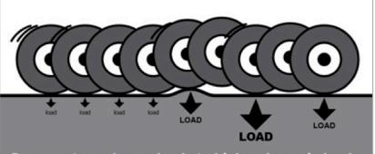
Pavement roughness leads to higher dynamic loads on localized pavement sections, which increases pavement deterioration and increases fuel consumption as well as lowering ride quality. This also leads to a cycle of escalating deterioration rates with increasing roughness severity.
