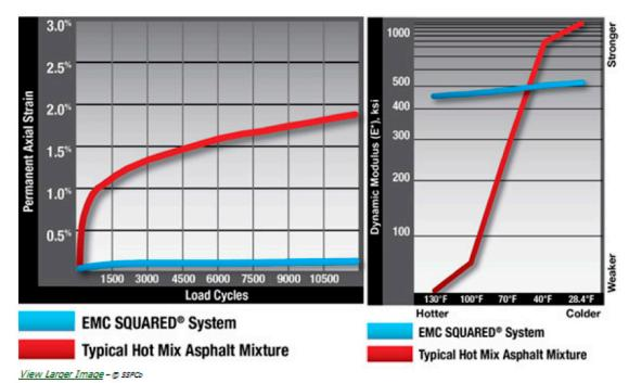
Left: Permanent deformation curves for Typical Hot Mix Asphalt mixture and an EMC SQUARED® stabilized aggregate mixture. Right: Typical Dynamic Modulus Data for Hot Mix Asphalt mixture and EMC SQUARED® stabilized aggregate mixture.
