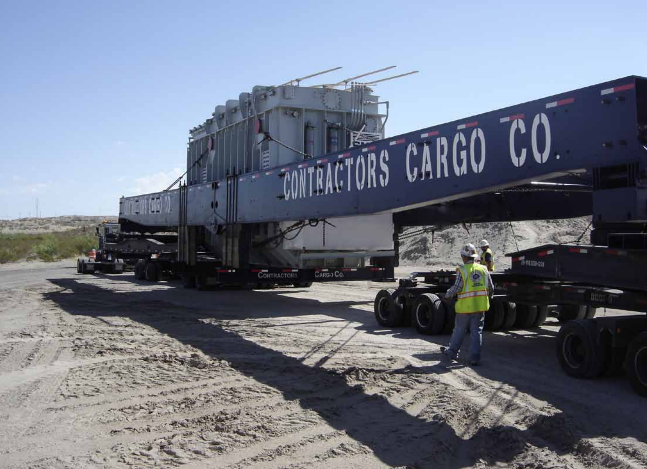
Stabilized Aggregate road bridging sand subgrade under heavy load as road detours around sand dune area.
