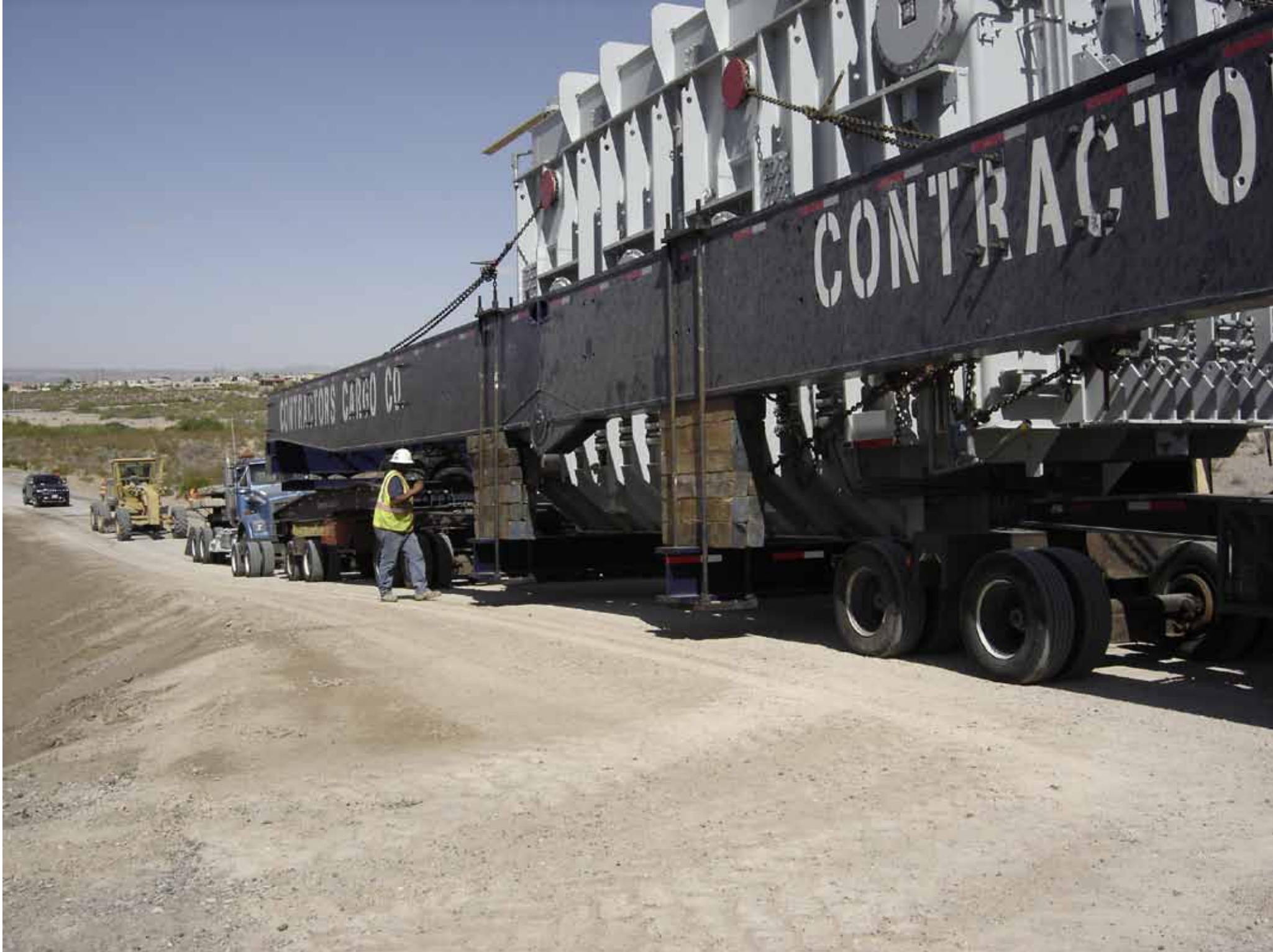
Heavy haul truck ascending grade with pusher truck in view at rear.
