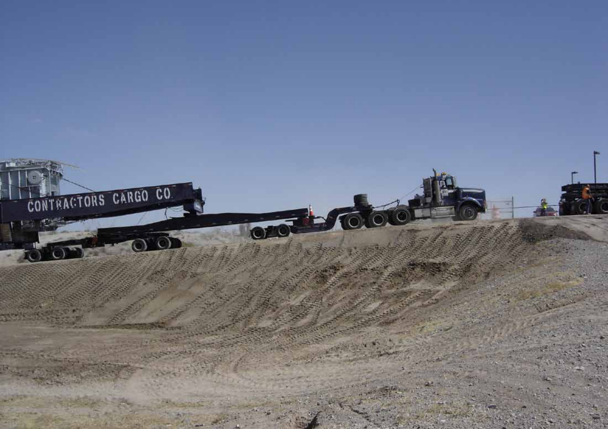
Primary haul truck cabled to puller truck as 200+ ton transformer is transported up steep grade.
