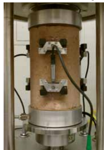
Stabilized Aggregate Sample in Dynamic Modulus testing Set-up
