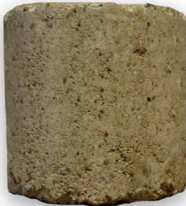
Recycled Aggregate Treated With EMC SQUARED Stabilizer (1000) (Test results at right)
