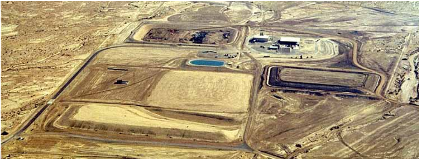
Aerial photo of hazardous waste disposal landfill facility in arid desert location. Final soil covers constructed with EMC SQUARED Stabilizer treatments approved by CalEPA for ongoing permanent closures as disposal cells are filled.
