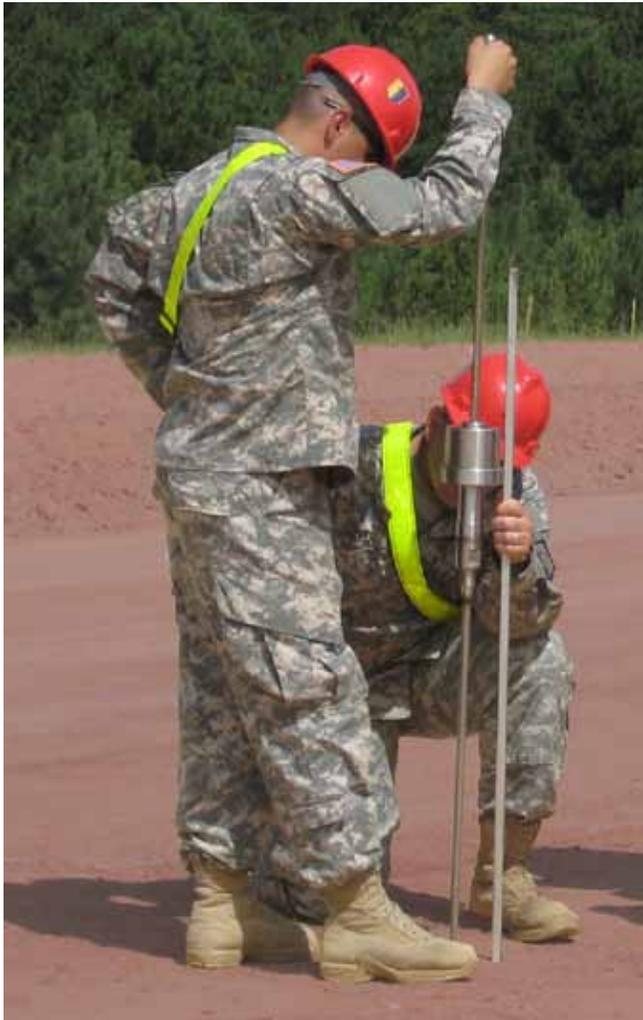
Field testing **EMC SQUARED** stabilized soil after initial curing by Penetrometer testing that measured a nearly seven-fold increase in bearing strength.
