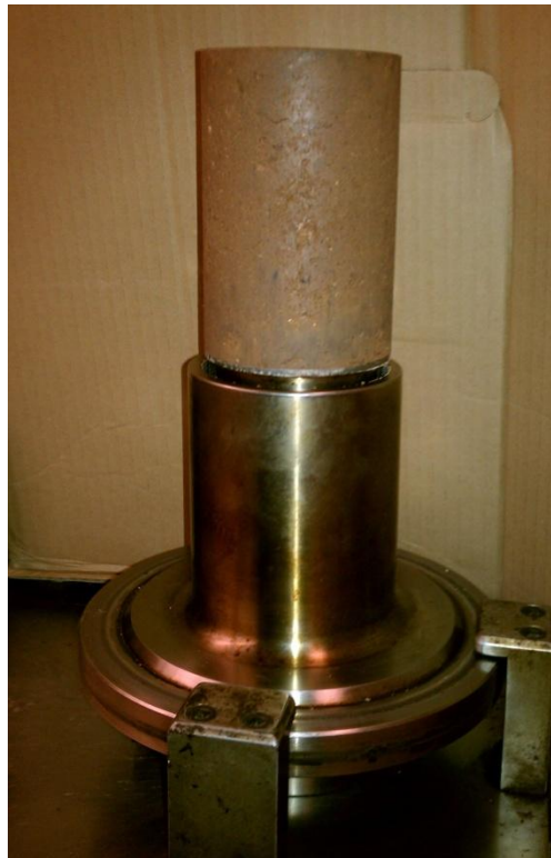
Figure 2. Compacted Sample of the Stabilized Aggregate Extruded from the SGC Mold.
