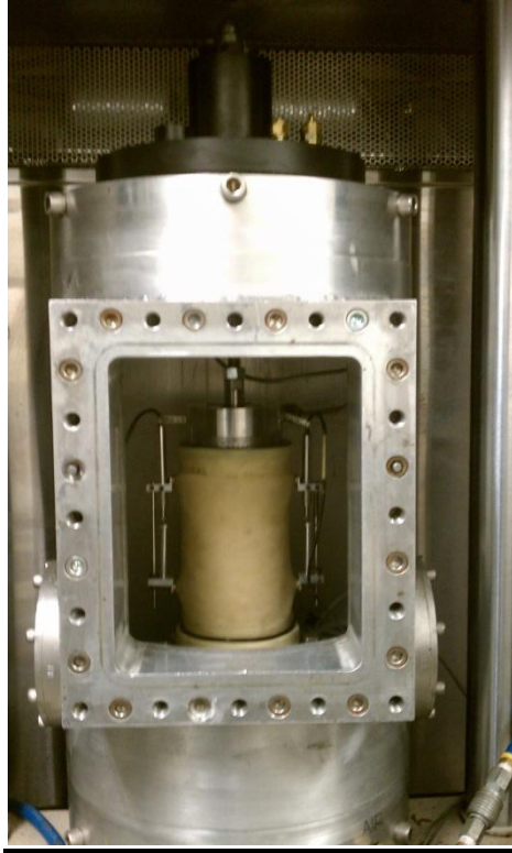
Figure 15. Stabilized Aggregate Sample in Repeated Load Triaxial testing Set-up.
