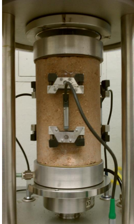
Figure 5. Stabilized Aggregate Sample in Dynamic Modulus testing Set-up.
