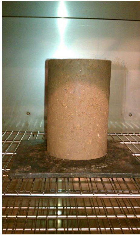
Figure 3. Compacted Sample of the Stabilized Aggregate Cured in Oven.
